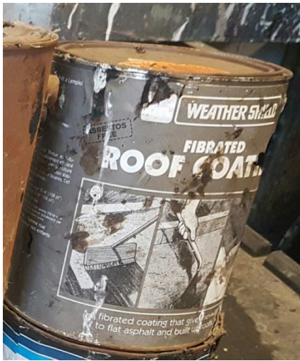
Roof tar, or repair
