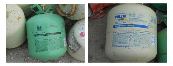
3. REFRIGERANT (FREON) TANKS – These tanks come in a number of colours and with a number of different label names (see below). These products can only be bought by licensed technicians and are **not accepted** at Product Care depots.
